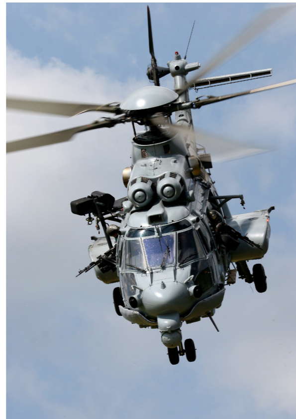
FN® airborne crew served weapon systems are equipped with FN MAG® or FN® M3M machine guns
