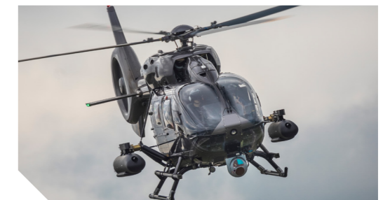
FN ® Pod systems on both sides of the helicopter, equipped with an FN ® M3M machine gun
